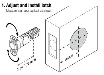
▲ If backset of door measures 2 3/4" (70mm), adjust latch by rotating face as shown.
