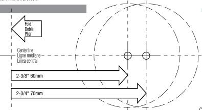
The drilling template must be printed to scale to ensure correct hole placement. To confirm correct print scale, the square below must measure exactly 1" by 1" (25mm x 25mm).
