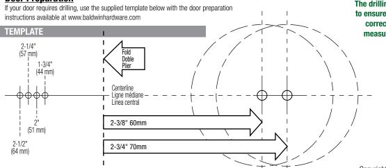
The drilling template must be printed to scale to ensure correct hole placement. To confirm correct print scale, the square below must measure exactly 1" by 1" (25mm x 25mm).
