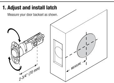
⚠ If backset of door measures 2 3/4" (70mm), adjust latch by rotating face as shown.
